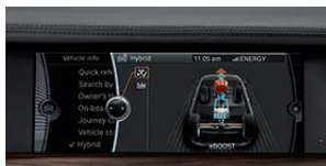
A clear graphic in the Control Display indicates the power flows in the vehicle in real time – electric power in blue, power from the combustion engine in red.
