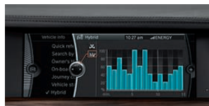
A bar chart in the BMW ActiveHybrid 7 indicates hybrid utilisation. The display is updated every 60 seconds and shows the last 15 minutes. The higher the bar, the greater the usage of the hybrid system and the associated fuel savings.
